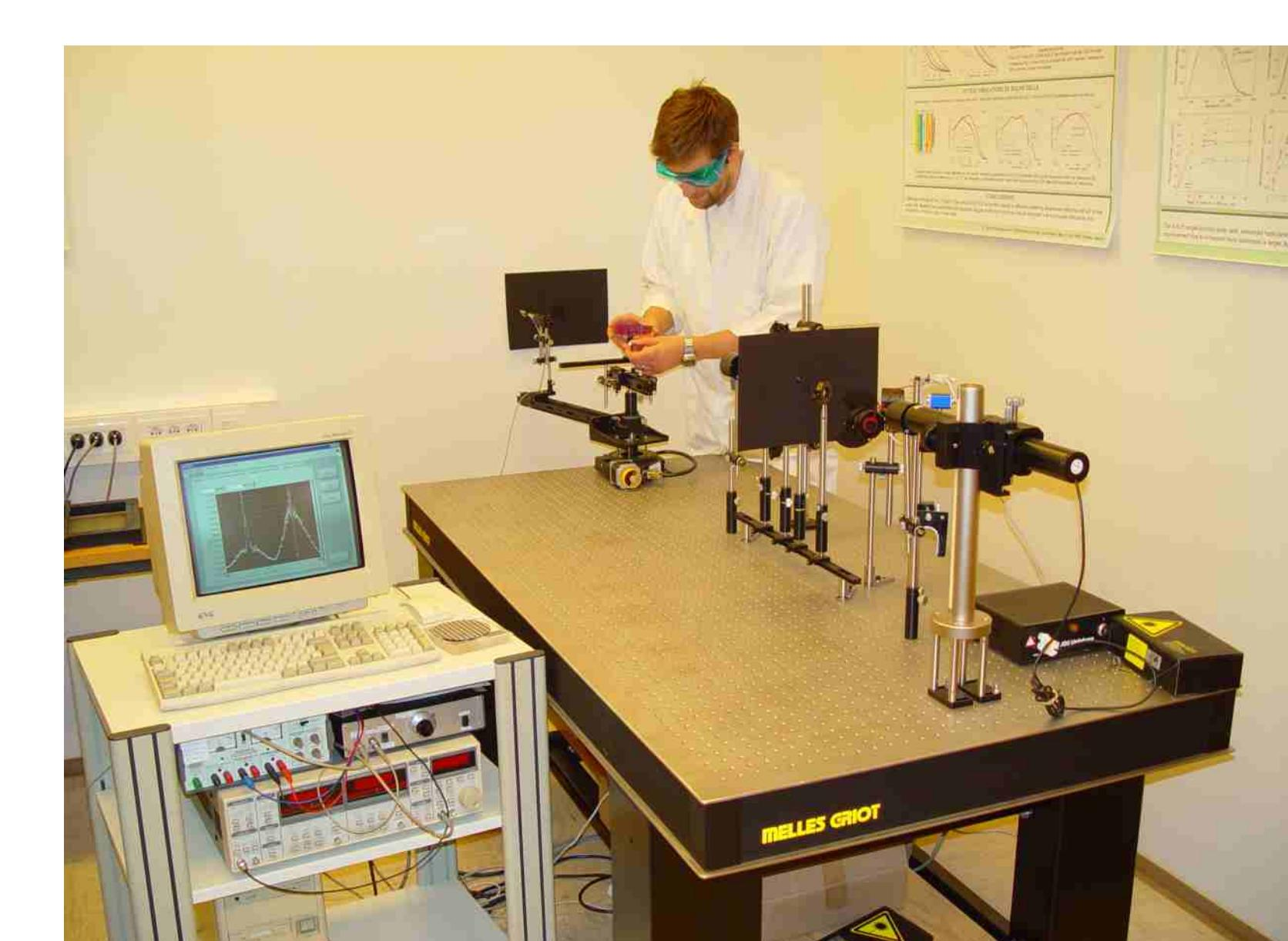
Angular resolved scattering measurement setup
