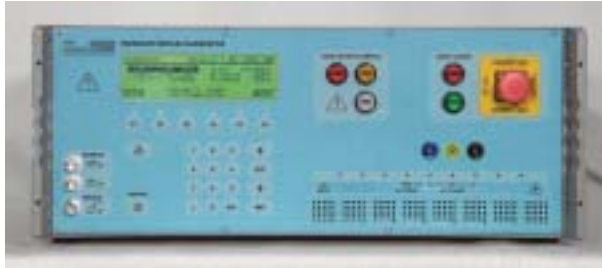
MIG0603IN4: Ring 100 kHz, 6.3 kV
