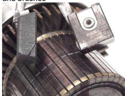
Figure 2-4. Commutator and brushes
