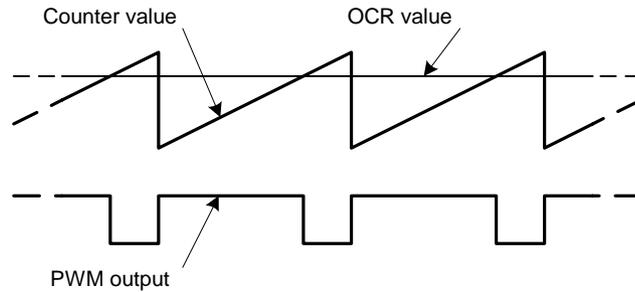
If using the high-speed PWM to generate analog signals, the step-size between the analog levels is depending on the resolution of the PWM. The higher base frequency the more easily is it to attenuate the base frequency and thereby minimize the signal ripple. The selection of resolution versus base frequency is thus an application dependent trade-off.
