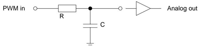
If the analog signal is fed to a low-impedance input, a buffer amplifier should be connected between the filter output and the load. This will prevent the load from discharging the capacitor and creating ripple voltages.
