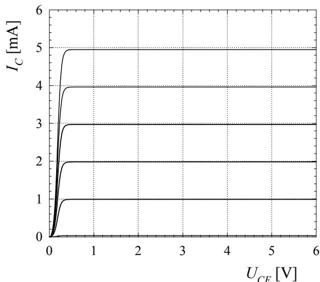
**(Rešitev:  $\beta_F = 99$ ,  $I_C = 3 \text{ mA}$ ,  $I_B = 30,3 \text{ } \mu\text{A}$ , tokovi: 0, 10, 20, 30, 40, 50  $\mu\text{A}$ )**
