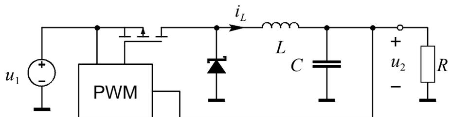
(Rešitev:  $I_2 = 5 \text{ A}$ ,  $U_1 = 28 \text{ V}$ :  $D = 0,439$ ,  $\Delta I_L = 2,34 \text{ A}$ ,  $I_{Lmax} = 6,17 \text{ A}$ )
