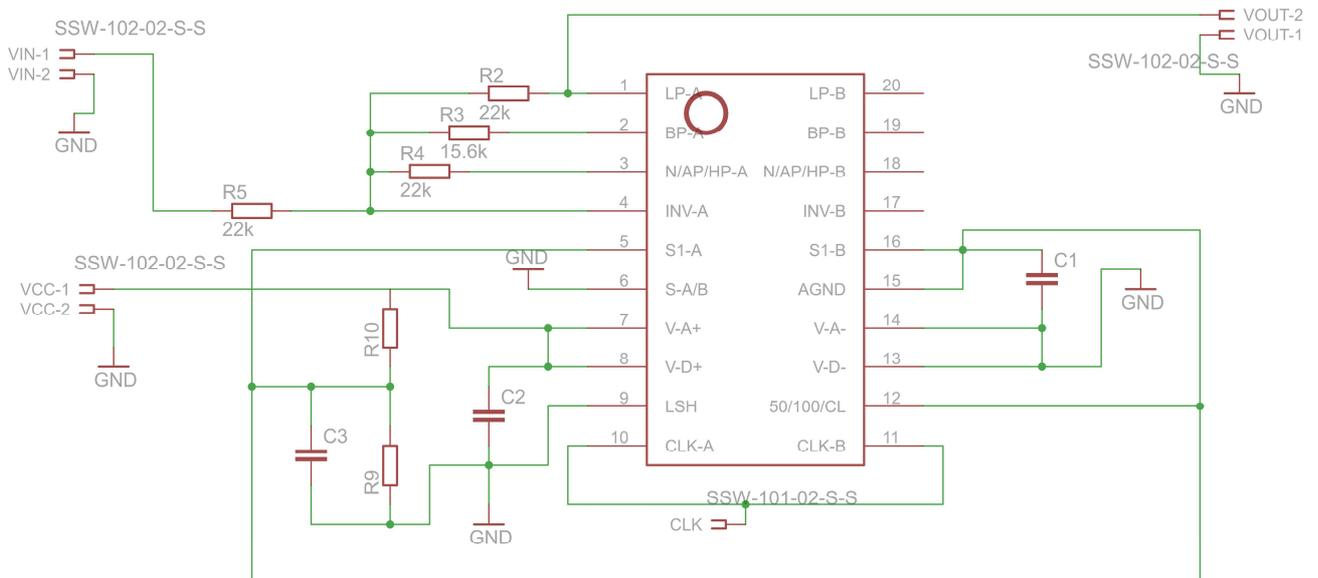
$$f_O = \frac{f_{CLK}}{100} \times \sqrt{\frac{R_2}{R_4}} \text{ or } \frac{f_{CLK}}{50} \times \sqrt{\frac{R_2}{R_4}}$$
