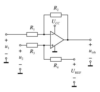
• Use the proposed circuit to generate reference voltage  $U_{\text{REF}} = 5 \text{ V}$ .
